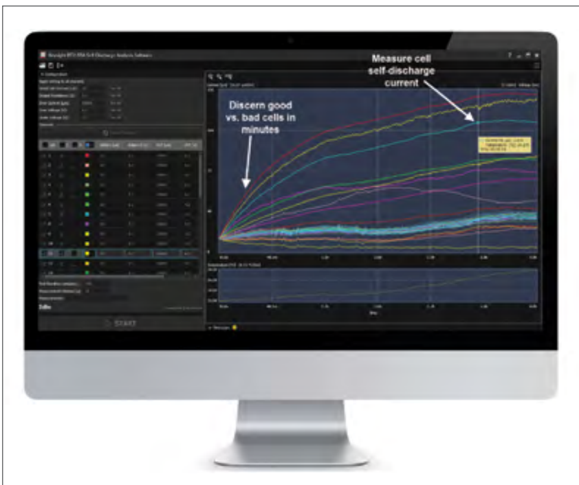
Figure 3: Results from a 4 hour test of 18650 cells using a high-performance potentiostatic analyser. Image: Keysight Li-Ion Self-Discharge Measurement Solutions.
