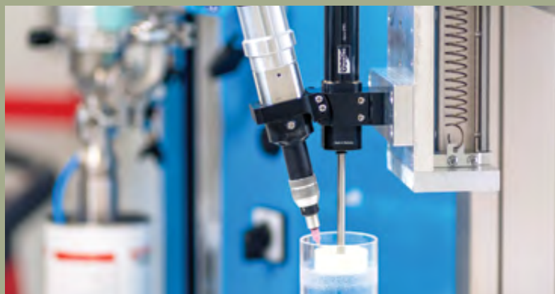
Rotorspray with RD dispenser during a spray test in the ViscoTec technical centre.
