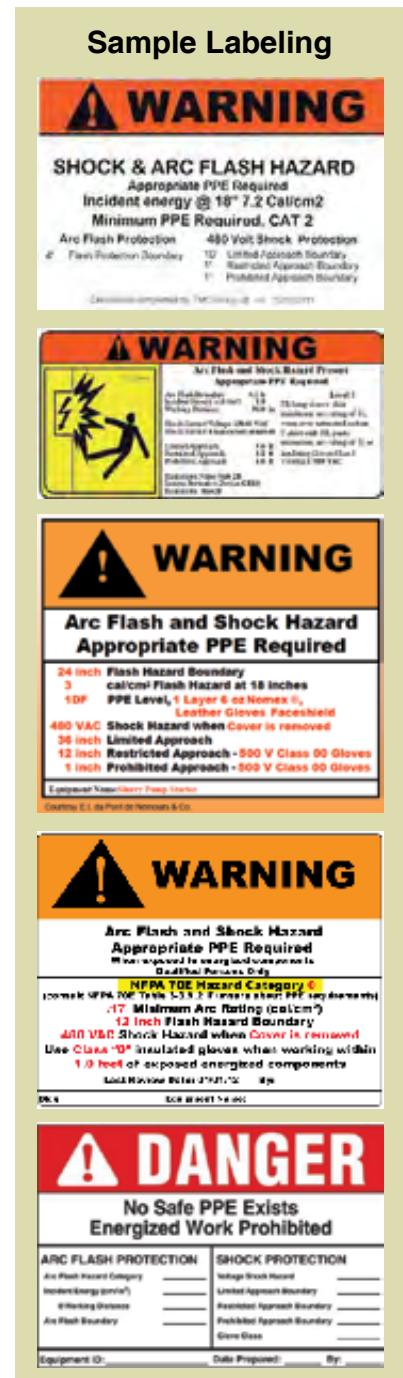
Arc flash hazard warning labels.
